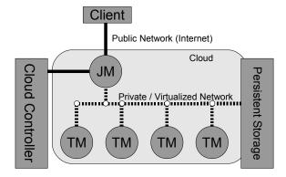
Fig. 1. Structural overview of Nephele running in an Infrastructure-as-a-Service (IaaS) cloud
