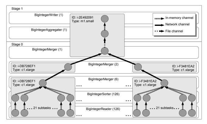
Fig. 6. The Execution Graph for Experiment 3 (DAG and Nephele)
