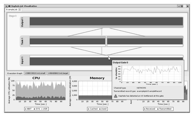
Fig. 4. Nephele's job viewer provides graphical feedback on instance utilization and detected bottlenecks
